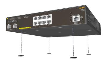
**2.** Position the switch firmly on the tabletop or desktop.
