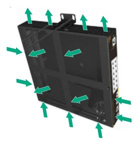
**Figure 19:** Aruba 2930F 12G airflow: Ports facing downward
