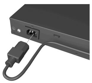
**b.** For Aruba 2930F 8G (JL258A, JL692A) switches, plug the power cord for the AC/DC adapter into the switch. Then plug the AC/DC power adapter into a nearby AC power source.
