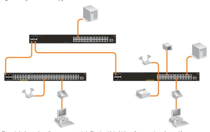
The switch also works well as a segment switch. That is, with its high performance, it can be used for interconnecting network segments. Simply connect the network devices that form those segments to the switch or you can also connect other switches.
