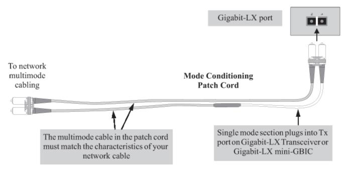
Be sure to purchase a patch cord that has appropriate connectors on each end, and has multimode fibers that match the characteristics of the multimode fiber in your network. Most important, the core diameter of the multimode patch cord must match the core diameter of the multimode cable infrastructure (either 50 or 62.5 microns).
