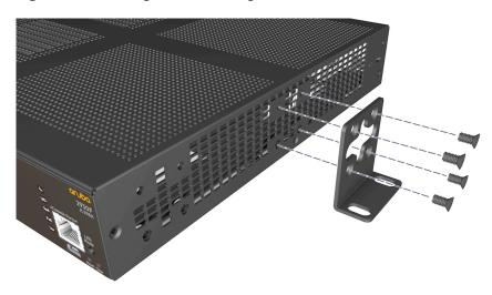
**2.** Attach the switch to the wall or under-table location using four 5/8-inch number 12 wood screws (not included).
